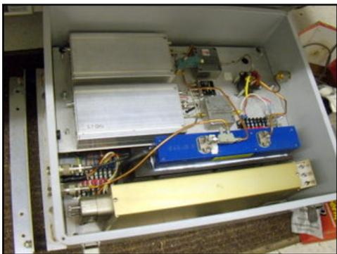
The feed is being prepared and it has a waveguide transition to a Chaparral feed to be mounted once the dish is out of the garage. The RF amplifier and power supply are contained in a large weather-proof box with both 5GHz and 10GHz amplifiers. These were obtained from N3FTI when he downsized his rover station. As we understand, the TWT is capable of at least 40W output.
